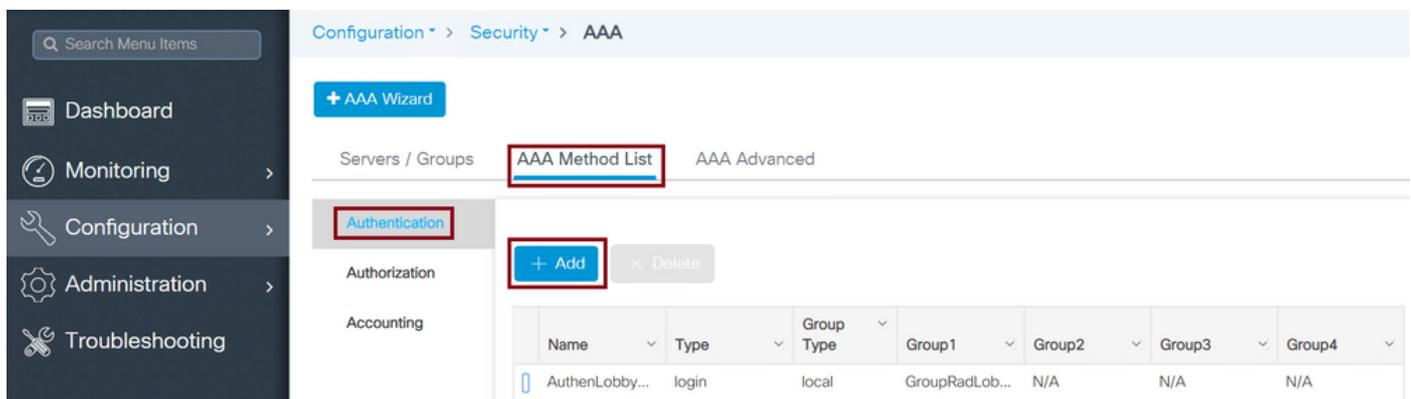
The screenshot shows the Cisco WLC GUI configuration page for AAA Method List. The breadcrumb path is Configuration > Security > AAA. The 'Authentication' tab is selected. A table lists the method 'AuthenLobby...' with type 'login' and group 'GroupRadLobby...'. A '+ Add' button is highlighted.
