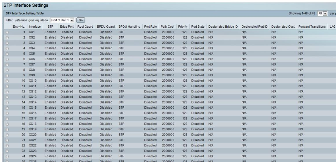
The screenshot shows the 'STP Interface Settings' page with a table titled 'STP Interface Setting Table'. The table has 16 columns: Entry No., Interface, STP, Edge Port, Root Guard, BPDU Guard, BPDU Handling, Port Role, Path Cost, Priority, Port State, Designated Bridge ID, Designated Port ID, Designated Cost, Forward Transitions, and LAG. There are 25 rows of data, each representing an interface from XG1 to XG25. All STP settings are 'Enabled', and all other settings are 'Disabled' or 'N/A'.
