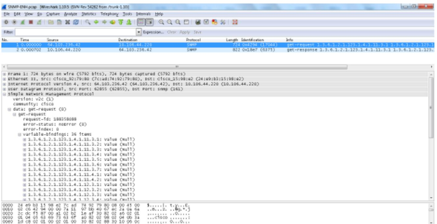
The image shows a Wireshark capture of an SNMP message. The packet list pane shows two packets: a get-request (packet 1) and a get-response (packet 2). The packet details pane shows the structure of the SNMP message, including the version (v2c), community (cisco), and the request data. The request data is a get-request for multiple MIB objects, and the response data is a get-response containing 36 variable bindings, all with null values.
