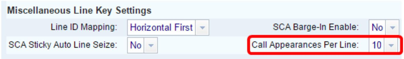
The screenshot shows a configuration panel titled "Miscellaneous Line Key Settings". It contains four dropdown menus: "Line ID Mapping" is set to "Horizontal First", "SCA Barge-In Enable" is set to "No", "SCA Sticky Auto Line Seize" is set to "No", and "Call Appearances Per Line" is set to "10". The "Call Appearances Per Line" dropdown is highlighted with a red rectangular box.
