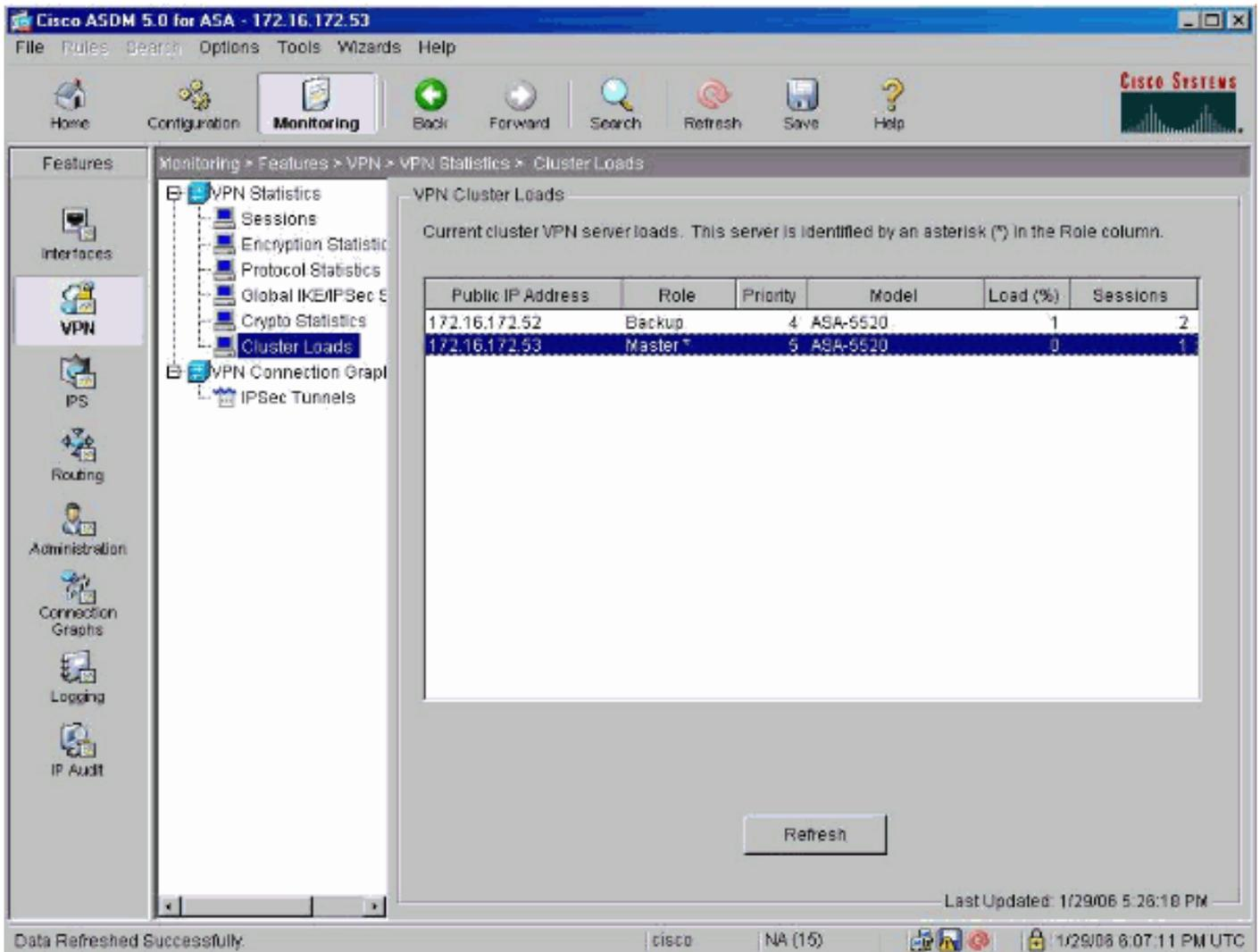
The screenshot displays the Cisco ASDM 5.0 for ASA interface. The breadcrumb navigation path is Monitoring > Features > VPN > VPN Statistics > Cluster Loads. The main content area shows the 'VPN Cluster Loads' configuration page. It includes a table with the following data:
