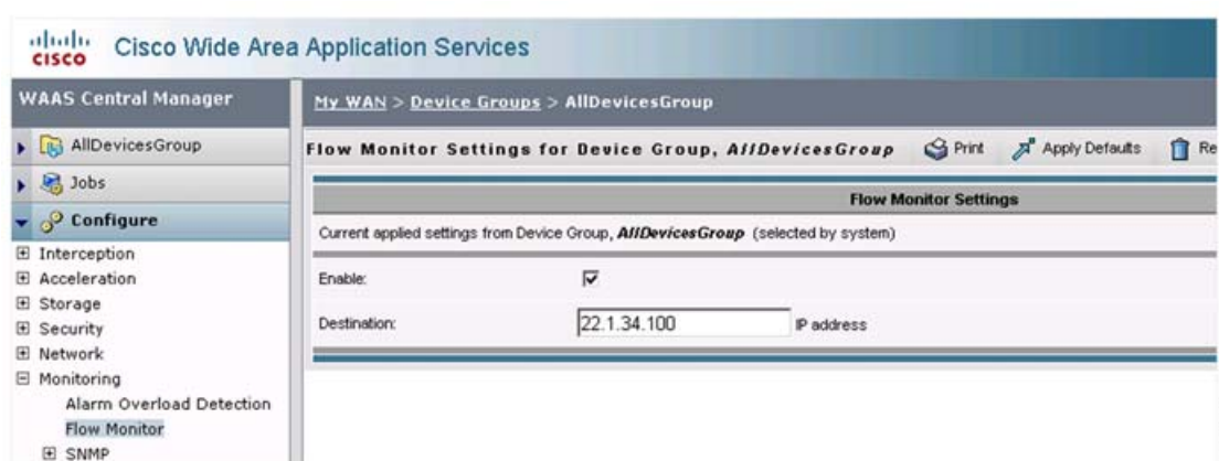
図 5-2 WAAS Central Manager : [Flow Monitoring Settings]
