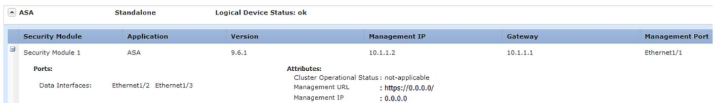
The screenshot shows the Chassis Manager interface for an ASA device. The device is in Standalone mode with Logical Device Status: ok. The configuration table is as follows:
