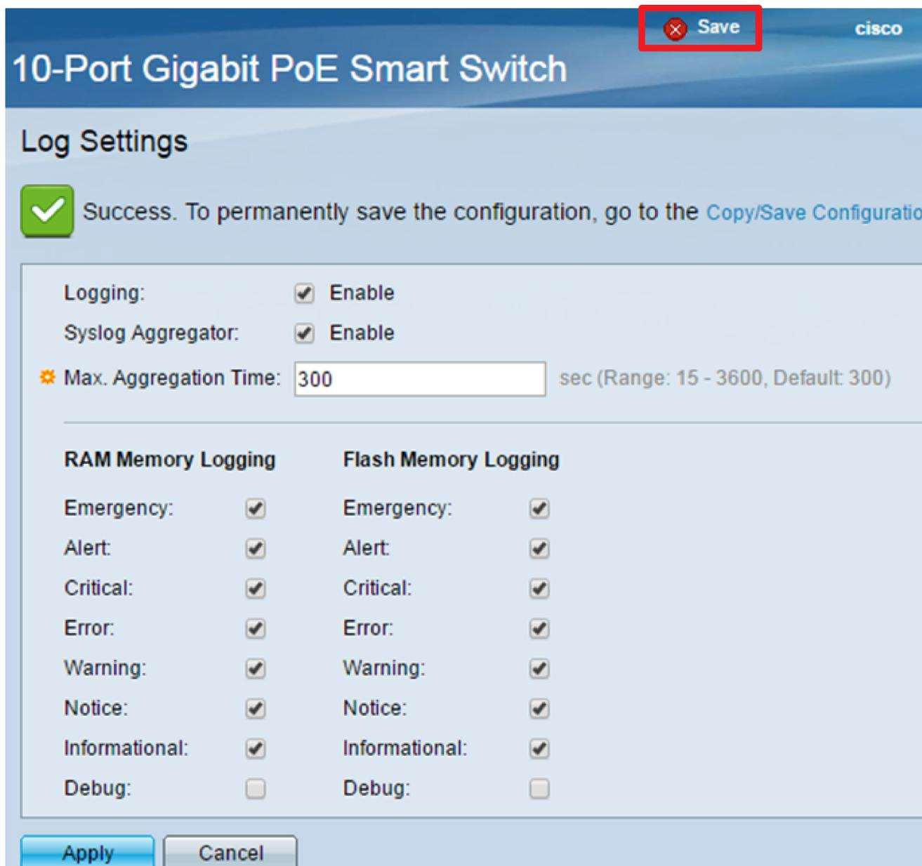
The screenshot shows the Cisco configuration interface for a 10-Port Gigabit PoE Smart Switch. The page title is "10-Port Gigabit PoE Smart Switch" and the section is "Log Settings". A "Save" button is highlighted with a red box. A success message is displayed: "Success. To permanently save the configuration, go to the [Copy/Save Configuration](#)". The configuration options are as follows:
