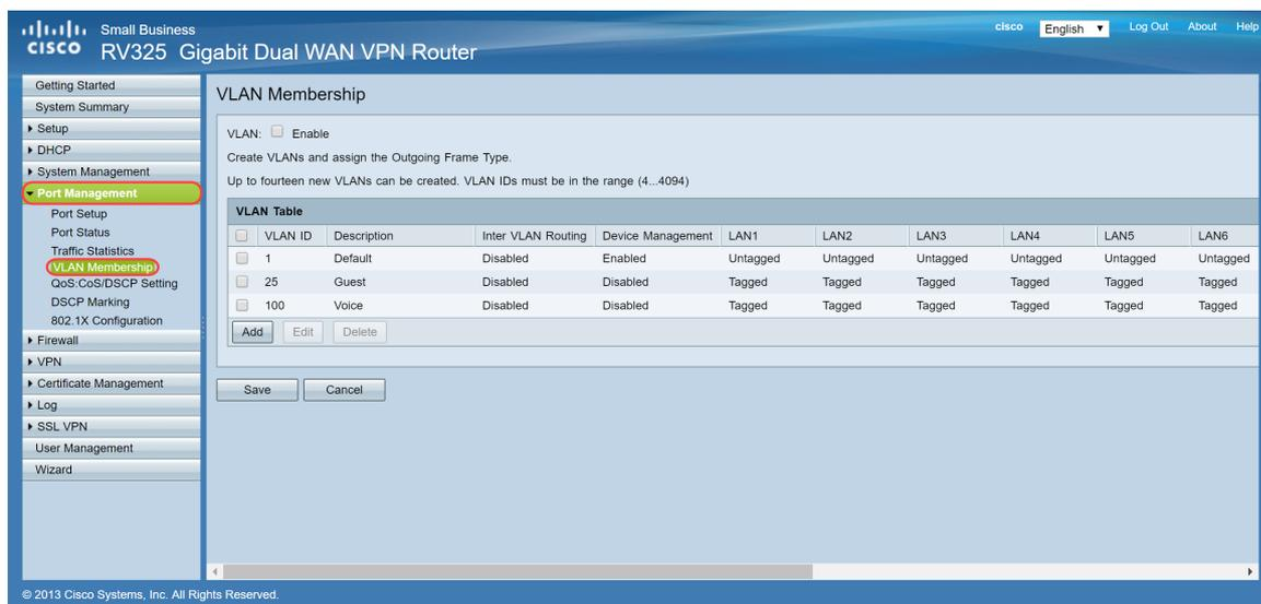
The screenshot shows the Cisco RV325 Web Management Interface. The left sidebar contains a navigation menu with 'Port Management' selected. The main content area is titled 'VLAN Membership' and includes a 'VLAN' checkbox which is currently unchecked. Below this is a table with the following data:
