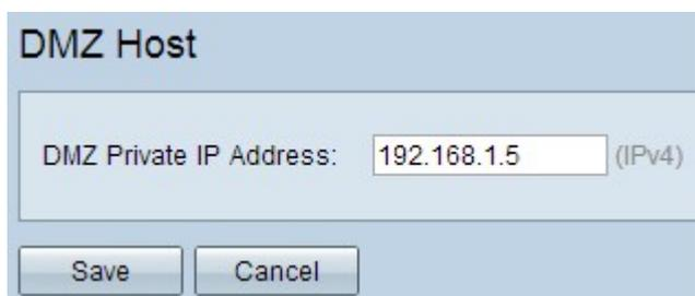
The screenshot shows the 'DMZ Host' configuration window with the IP address '192.168.1.5' entered in the 'DMZ Private IP Address:' field. The '(IPv4)' label is still present to the right of the field. The 'Save' and 'Cancel' buttons are at the bottom.
