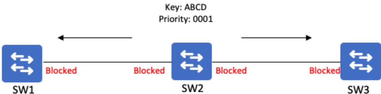
2. Receive BPA with key and higher priority from SW1 causing port to go OPEN
