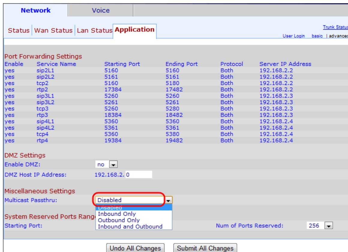
The screenshot shows the 'Application' configuration page in the SPA8000 web interface. The 'Multicast Passthru' dropdown menu is open, and the 'Disabled' option is highlighted with a red circle. The page also displays 'Port Forwarding Settings' and 'DMZ Settings'.
