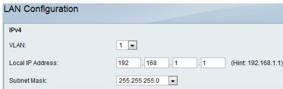
The screenshot shows the 'LAN Configuration' web utility. Under the 'IPv4' section, there are three fields: 'VLAN' with a dropdown menu set to '1', 'Local IP Address' with four input boxes containing '192', '168', '1', and '1' (with a hint '(Hint: 192.168.1.1)'), and 'Subnet Mask' with a dropdown menu set to '255.255.255.0'.
