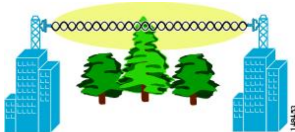
Figure 16: Typical Obstructions in a Fresnel Zone
