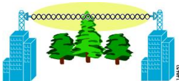
Figure 16: Typical Obstructions in a Fresnel Zone
