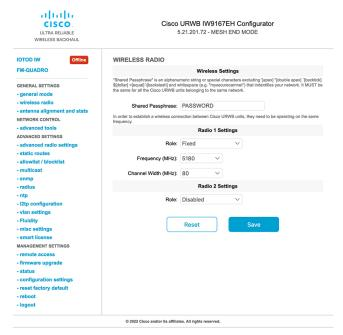
2. Set Radio 1 operating mode(role) as a Fluidmax Primary with FluidMAX Cluster ID. In this case the frequency selection on the Primary will be enabled and Secondary will be disabled. Select the maximum power level (power level 1 sets the highest transmit power) and Cisco URWB transmission power control (TPC) will automatically select the optimum transmission power.
