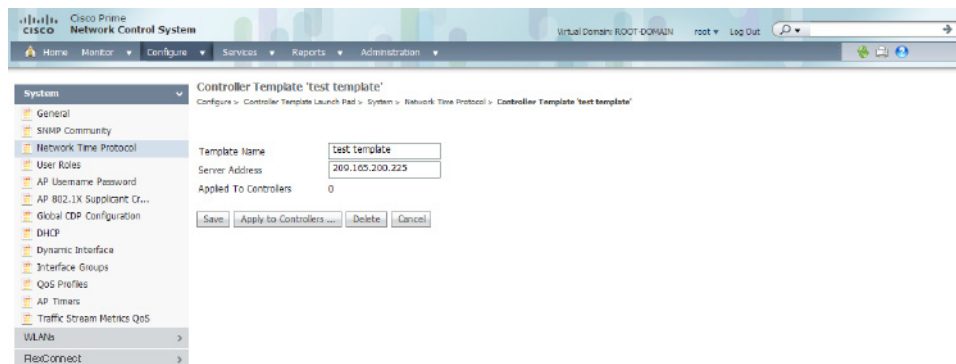
Figure 11-2 NTP Servers Template
