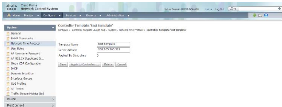
Figure 10-2 NTP Servers Template
