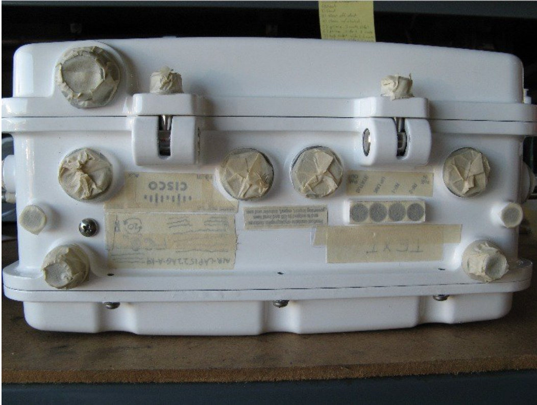
Figure 5: When painting do not get paint into any of the connectors (tape them properly)
