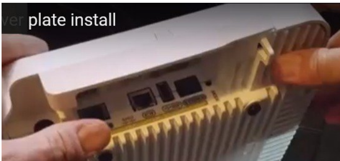
Figure 4: Example of a 3D printed cover installed
