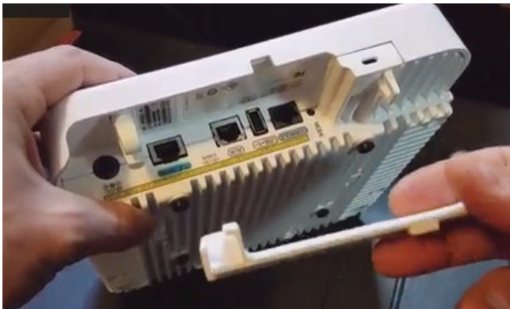
Figure 4: Example of a 3D printed cover installed
