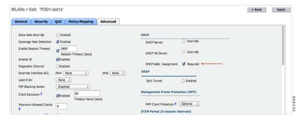
2. After enabling the DHCP required option, scroll down and in the **Local Client Profiling** area, enable DHCP Profiling and HTTP Profiling if they are not enabled and click **Apply**.
