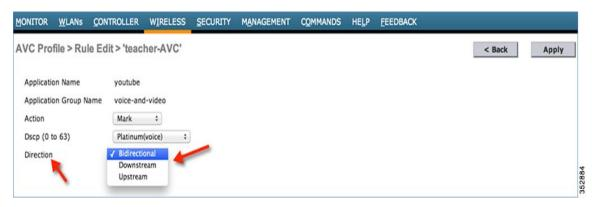
**5.** Once the appropriate Marking is selected, click **Apply**. The action rule will be created and is displayed as captured in the below screen. You can add more rules under the same AVC profile on the same page. A maximum of 32 rules can be configured in a single AVC profile.
