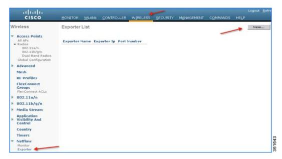
2. Enter the details of PAM, Exporter IP, as an example below 10.10.105.3 and Port Number as 9991 which will collect all the NetFlow stats generated by the WLC and then click **Apply**.
