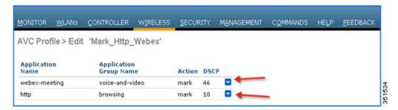
**Note:** For the same AVC profile two rules are created. The Administrator can configure up to 32 rules in the same AVC profile. Individual rules can be configured for action MARK or DROP in the same profile. A single rule can only be configured with a single action i.e. either MARK or DROP.
