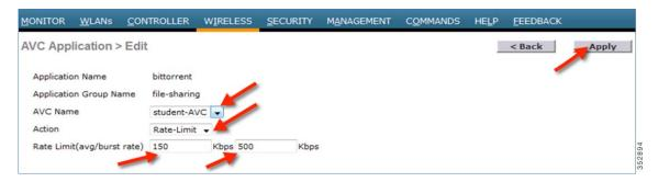
The BitTorrent application displays ratelimit in the Action column with Rate Limit average and burst rate values.
