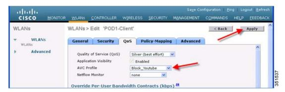
**Note:** If Application visibility is not enabled on the WLAN, and users selects an AVC profile and Apply is clicked, this automatically enables Application visibility. But to disable Application visibility from WLAN, AVC profile, which is mapped to WLAN, should be removed first by selecting **None** from drop-down.
