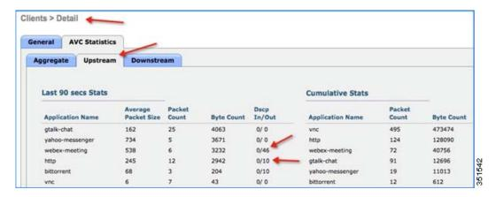
Notice the above output and make sure the WebEx application is getting OUT DSCP value as 46 because the WebEx application is been configured with Platinum QOS profile and HTTP application is getting OUT DSCP value as 10 because the HTTP application is been configured with Bronze profile.
