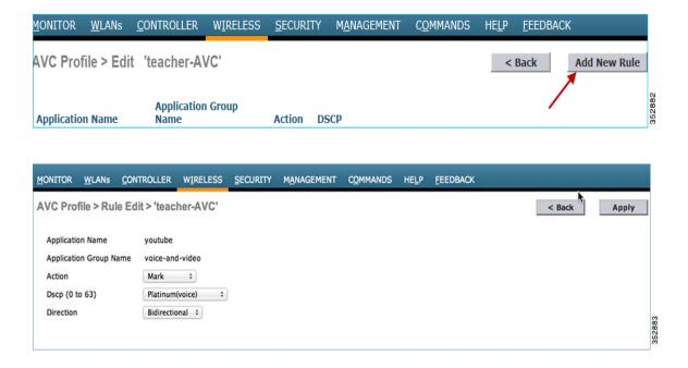
**Note:** WLC is capable of classifying 1105 applications with Protocol Pack 11.0 and gives an option to take action. To take an action on any application, the administrator has to select the application group first to which that application belongs, which will filter the list of applications for that application group only. The reason for this implementation is all 1105
