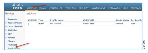
Now click the individual WLAN ID and the below screen will be visible which will list aggregate data for the top ten applications running on that particular WLAN.
