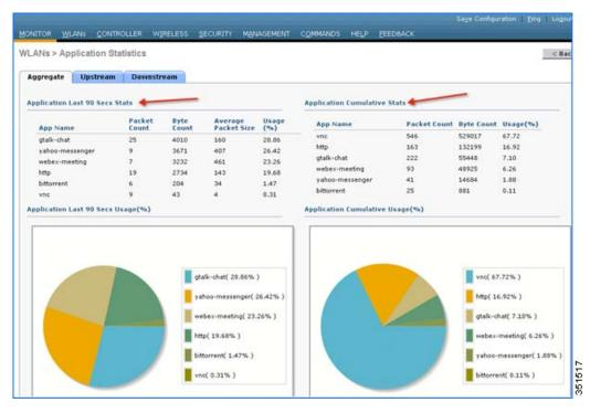
**Note:** This page will provide more granular visibility per WLAN and will list the top ten applications in last the 90 seconds, as well as cumulative stats for the top ten applications. The above screen lists the aggregate traffic on a particular WLAN, which includes upstream as well as downstream data. You can view UPSTREAM and DOWNSTREAM stats individually per WLAN from same page by clicking the **Upstream** and **Downstream** tab.
