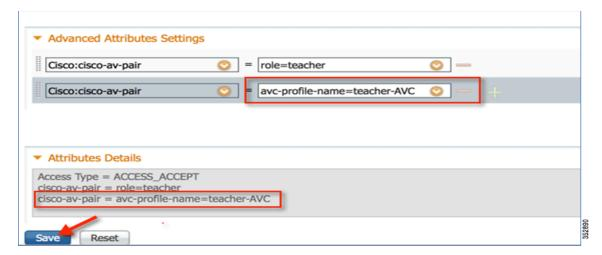
If you are using the Cisco ACS, go to **Policy Elements > Authorization and Permissions > Network Access > Authorization Profiles.** Add **cisco-av-pair** to match the string value **avc-profile-name=***The AVC profile name created on the WLC.*
