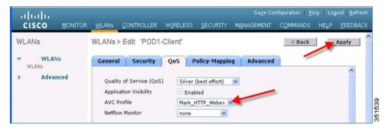
15. Once the AVC profiles are applied on the WLAN, it is also visible under **Monitor > Applications**. All the WLANs which has Application Visibility enabled will be displayed.
