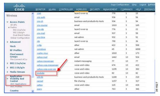
8. After Apply is clicked, the action rule will be created and displayed as captured in the below screen. You can add more rules under the AVC profile on the same page. Maximum of 32 rules can be configured in a single AVC profile.
