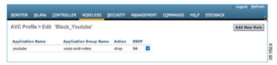
9. Another rule can be configured under the same AVC profile to MARK traffic with a different QOS profile or custom DSCP value. In this example, another AVC profile was created following step 3, 4 and 5 with the name "Mark\_Http\_Webex". In this example this AVC profile is used to create a rule to mark "Http" with low priority and give "Webex" more precedence.
