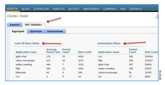
**Note:** This page will provide further granular stats per client associated on WLAN on which Application Visibility is enabled and will list the top ten applications in last 90 seconds as well as cumulative stats for top ten applications. The above screen lists the aggregate traffic per client, which includes upstream as well as downstream stats. You can view UPSTREAM and DOWNSTREAM stats individually per client from same page by clicking the **Upstream** and **Downstream** tab.
