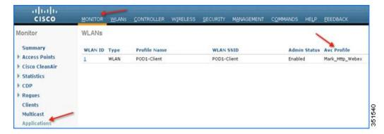
16. Once the AVC profile Mark\_Http\_Webex is applied on the WLAN, initiate or login to your individual WebEx account (if you have one) and also initiate some HTTP connections and observe the marking for these two applications under client details. Once the AVC profile is mapped to a WLAN and if it has a rule for the MARK action, that application will get precedence as per QoS profile configured in AVC rule overriding the QoS profile configured on the WLAN.
