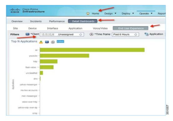
13. To see application usage per WLAN, navigate to Home > Detail Dashboards > End User Experience > Under Filter and then select the Network Aware as WLAN i.e. POD1-Client in this example. Click GO.
