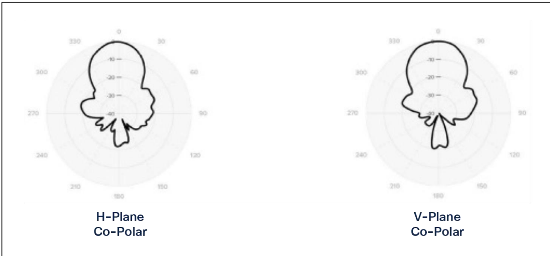
Figure 72. Meraki MA-ANT-F6 patterns at 2.4 GHz
