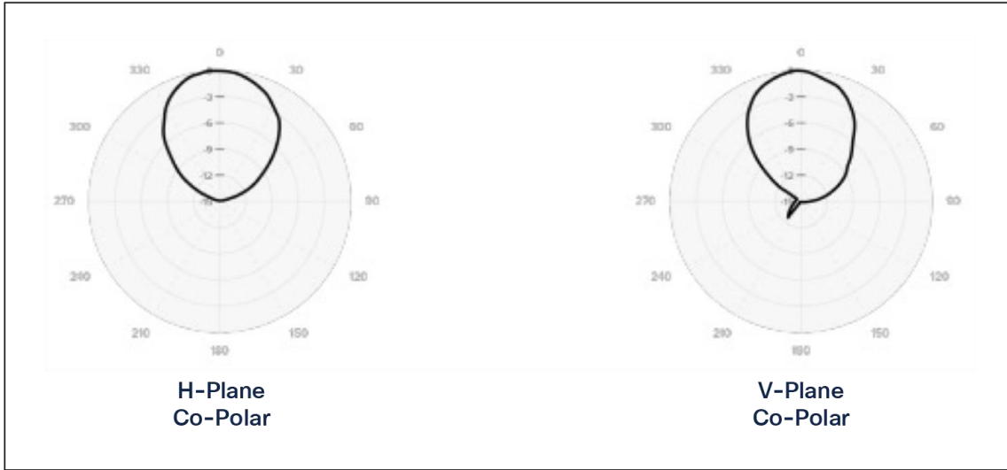
Figure 68. Meraki MA-ANT-E6 patterns at 2.4 GHz
