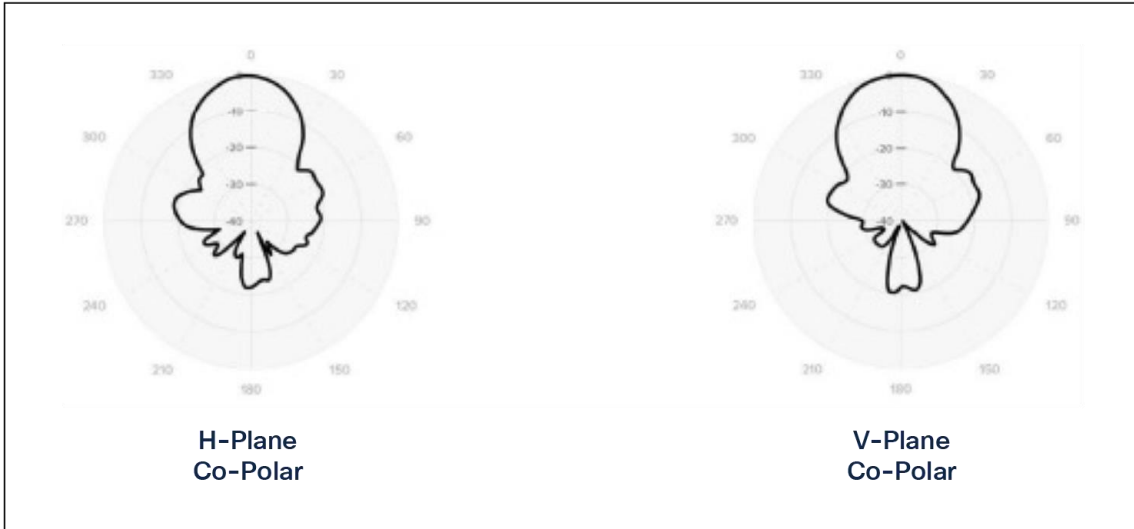
Figure 70. Meraki MA-ANT-F5 patterns at 2.4 GHz
