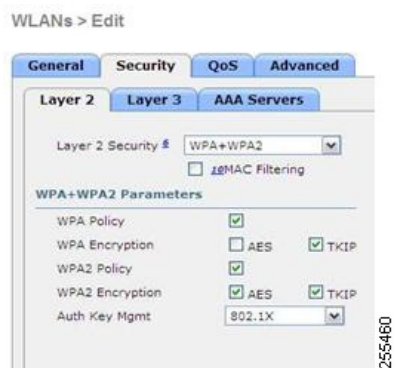
Figure 6: Incompatible WPA and WPA2 Security Encryption Settings for OEAP 600 Series
