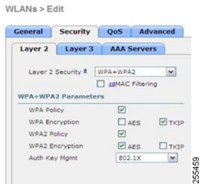
Figure 6: Incompatible WPA and WPA2 Security Encryption Settings for OEAP 600 Series
