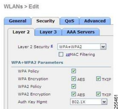
Figure 7: Compatible Security Settings for OEAP Series
