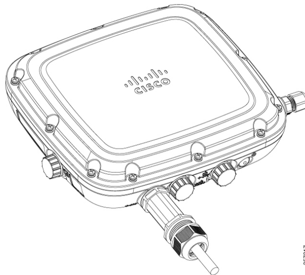
Figure 32: Fiber-Optic cable and gland installed to AP
