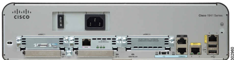
Figure 5 Interface Card and Service Module Configuration On a Cisco 1941 Router
