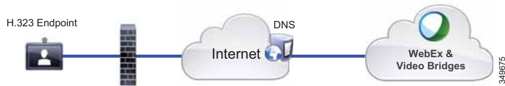
Figure 11-33 Cisco WebEx Meeting Center Video Conferencing Architecture Using H.323 Video Without Call Control System
