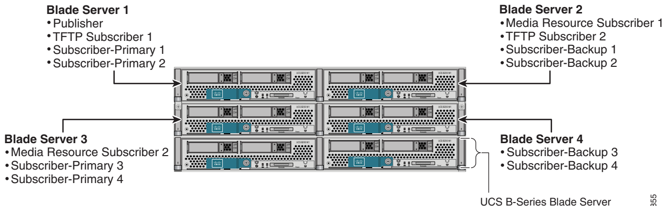
Figure 8-8 Unified CM Server Node Distribution on UCS
