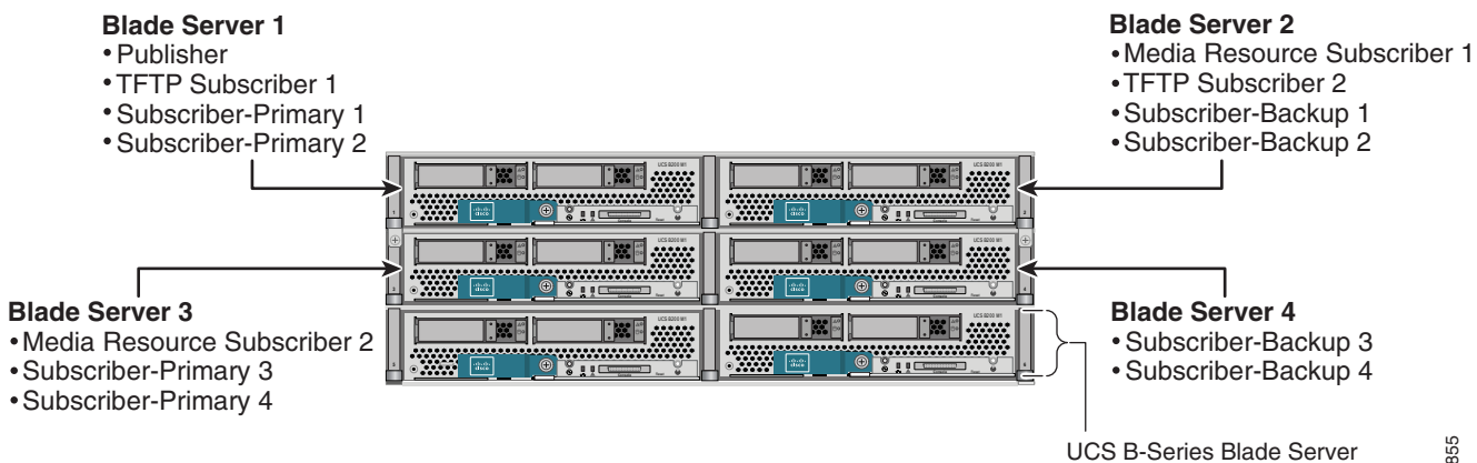
Figure 8-8 Unified CM Server Node Distribution on UCS
