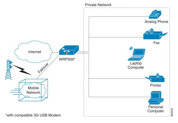
In this example, the business has the same network as illustrated in the "WRP500 Deployment in a Basic Network" section on page 1-3. However, this business has the added benefit of using the mobile broadband network as a backup network to ensure continuous Internet connectivity. In the event that the Internet connection fails, the WRP500 fails over to the configured mobile network. When the Internet connection becomes available, the WRP500 recovers the connection.
