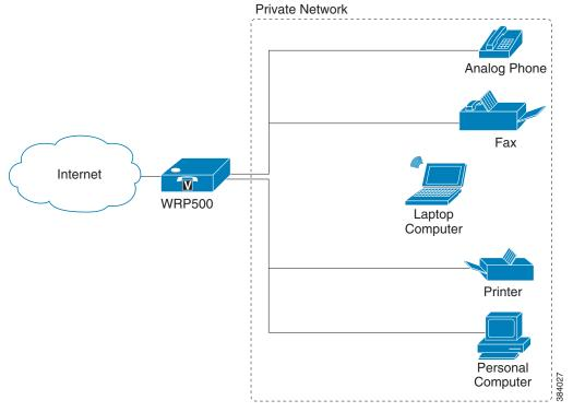
In this scenario, the WRP500 is deployed in a small business that has a basic network configuration.
