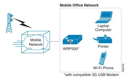
In this example, a team has set up a temporary network at a construction site. Team members have laptop computers and Wi-Fi phones that share a mobile broadband connection for Internet access. All computers can connect to the printer on the local network. If a Virtual Private Network (VPN) tunnel is configured on the laptop computer, team members also can securely connect to resources at the main office (not illustrated).
