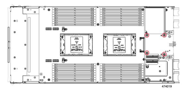
**Step 6** Using a T8 screwdriver, remove the screws on the sidewall.
