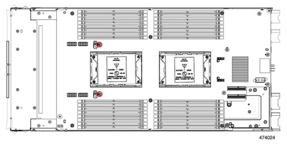
**Step 9** Using a T10 screwdriver, remove the Torx screws that secure the secondary PCB to the midframe.
