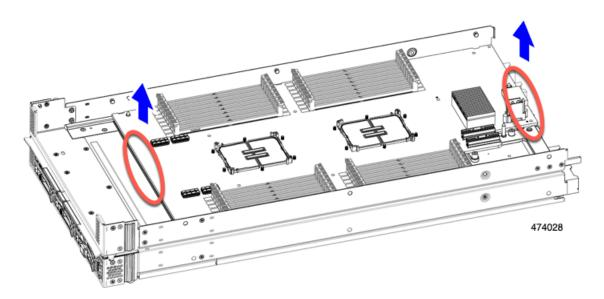
Step 12 Using a T10 screwdriver, remove the two screws that secure the primary's PCB to the midframe.
