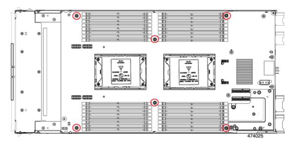
**Step 10** Using a T20 screwdriver, loosen the captive Torx nuts that hold each CPU bolster plate, then remove the plates. There are six nuts for each plate.
