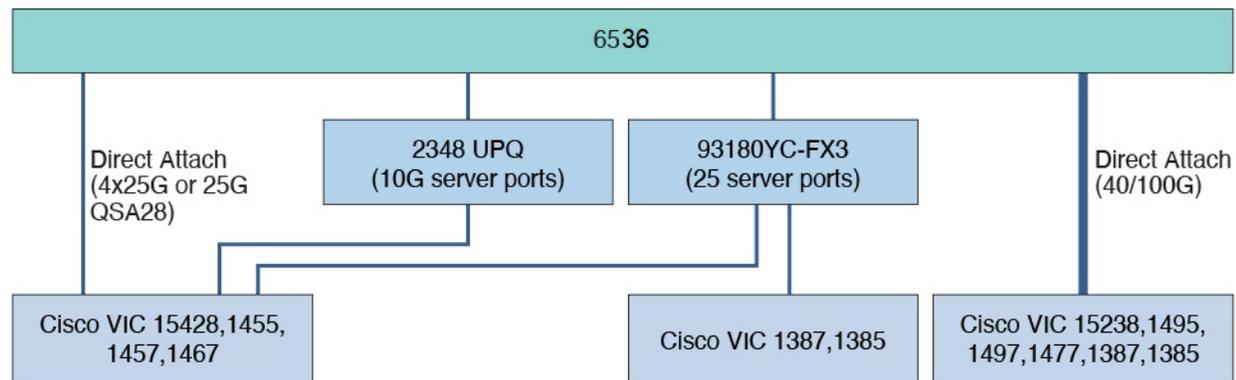
Figure 2: Network Topology for 6200, 6300, and 6400 Series Fabric Interconnect with 1300/1400/15000 Series VIC Cards
