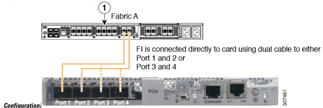
XGb represents a 40 Gigabit Ethernet connection or a 10 Gigabit Ethernet connection. For the 10 Gigabit Ethernet, the following cables are used:
