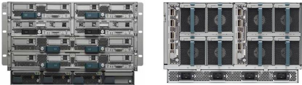
Figure 5 Cisco UCS 5108 Blade Server Chassis
