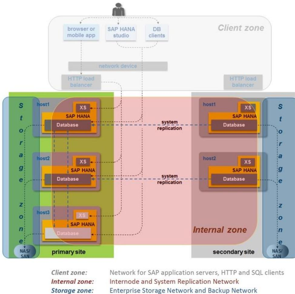
Based on the listed network requirements, every server must be equipped with 2x 10 Gigabit Ethernet for scale-up systems to establish the communication with the application or user (Client Zone) and a 10 GbE Interface for Storage access.
