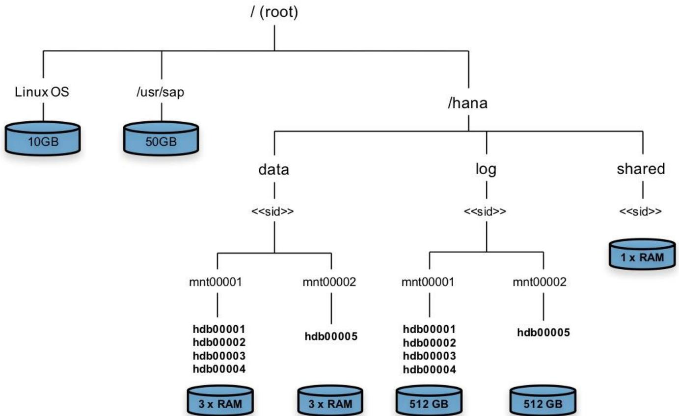
The storage sizing for filesystem is based on the amount of memory equipped on the SAP HANA host.
