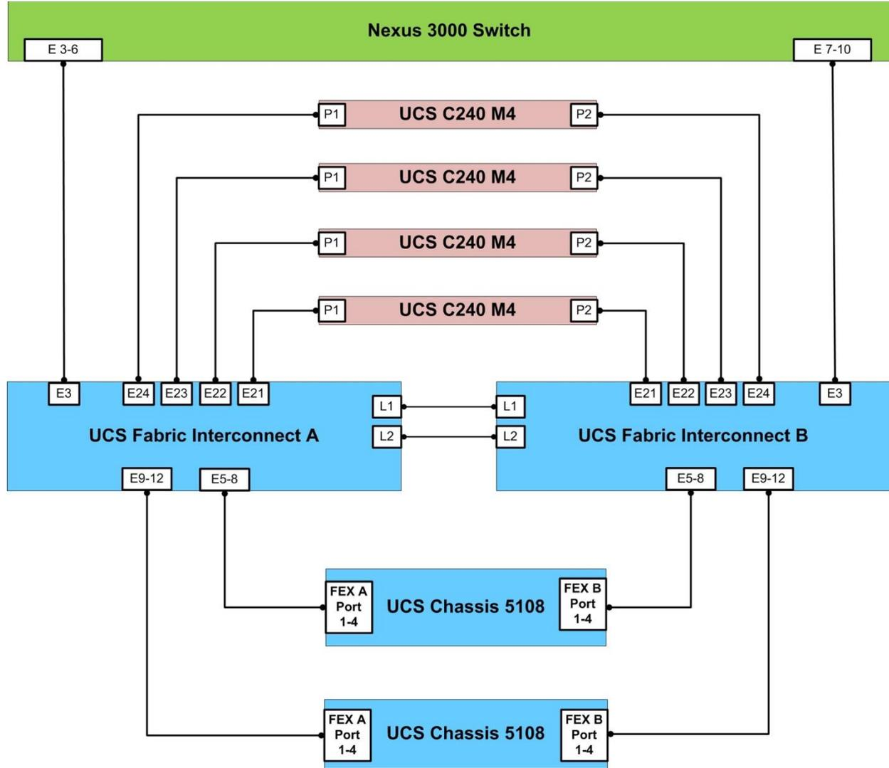
Figure 16 Cisco UCS Integrated Infrastructure for SAP HANA Configuration using the Cisco Nexus 3000
