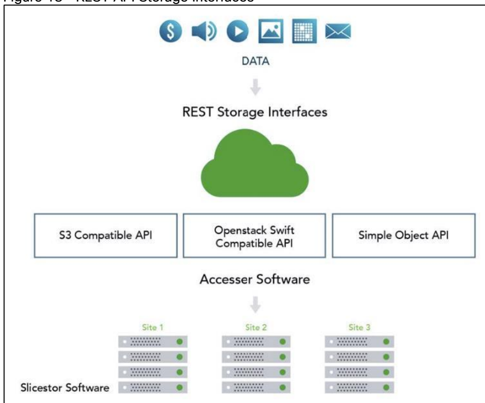
Figure 18 REST API Storage Interfaces
