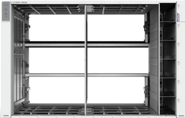
Figure 5. Cisco UCS X9508 Chassis - only power distribution midplane
