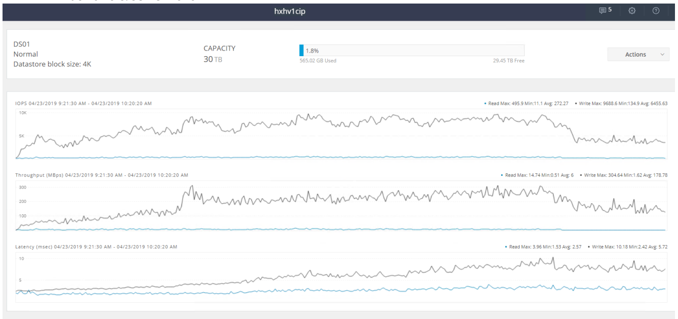
Figure 118 HyperFlex Cluster UI Performance Chart for Knowledge Worker Workload Running 200 User Test on Citrix Windows 10 & Server 2016.
