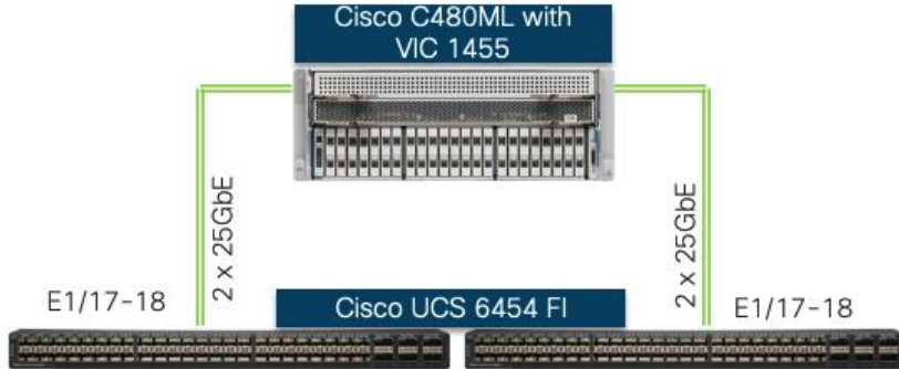
Figure 16 Cisco UCS C480 ML M5 to Cisco UCS 6454 FI Connectivity
