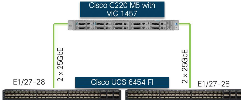
Figure 14 Cisco UCS C220 M5 to Cisco UCS 6454 FI Connectivity
