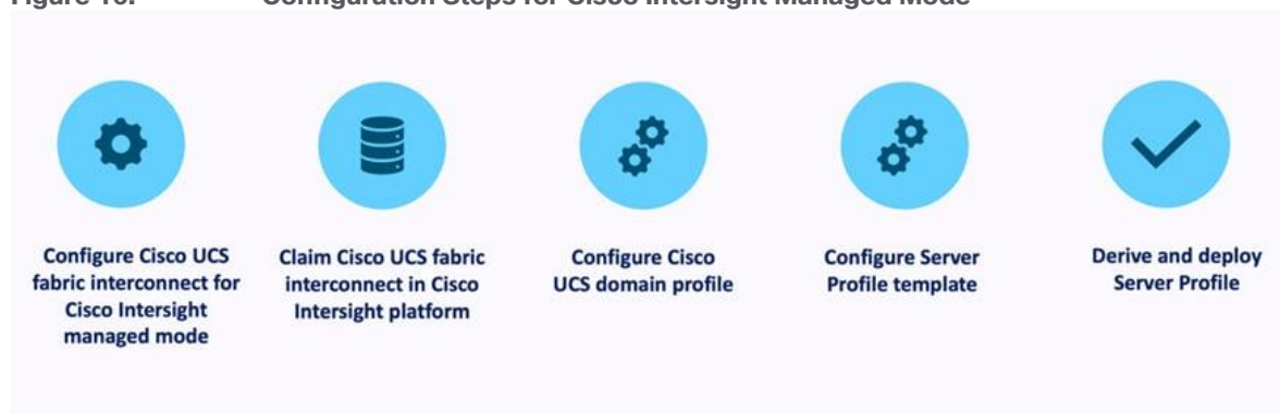
Figure 16. Configuration Steps for Cisco Intersight Managed Mode
