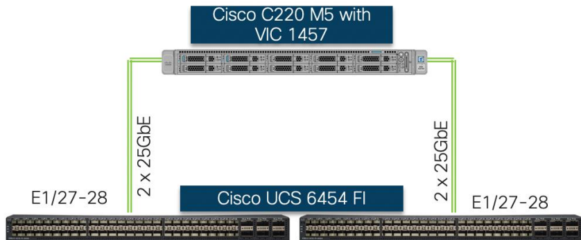
Figure 16 Cisco UCS C220 M5 to Cisco UCS 6454 FI Connectivity
