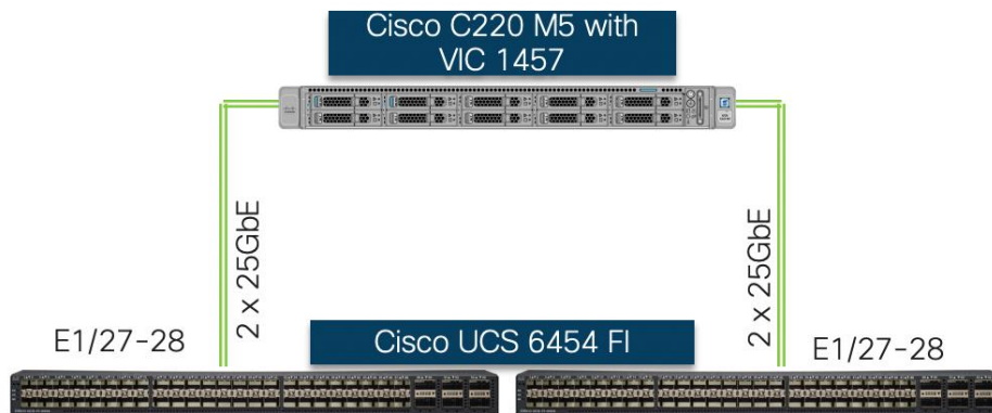
Figure 8 Cisco UCS C220 M5 to Cisco UCS 6454 FI Connectivity
