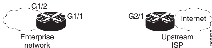
Figure 36-3 Enterprise Network Using Unicast RPF for Ingress Filtering
