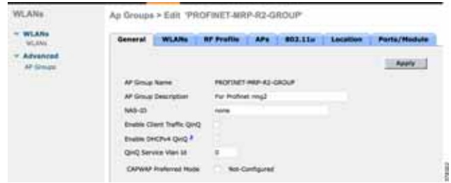
Figure 44 Create Access Point Group on WLC
