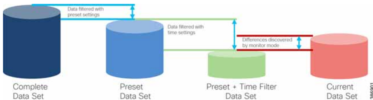
Figure 33 Baseline and Anomaly Detection by Cyber Vision
