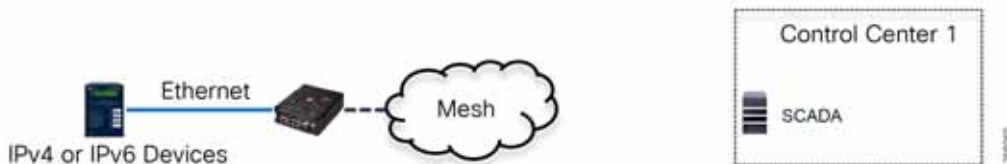
Figure 60 Edge Compute Application Connectivity
