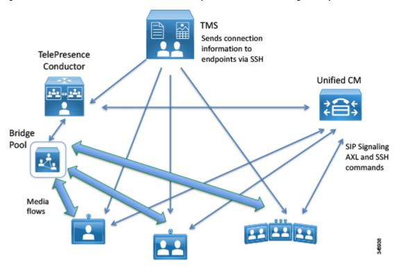
Figure 5-10 Cisco TMS Communicates Directly with Unified CM Managed Endpoints
