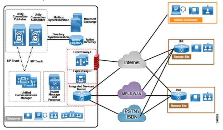
At the remote branch site, Cisco Unified Survivable Remote Site Telephony (SRST) is installed as a backup call agent, which is integrated with the central Unity Connection server. In the event of an IP WAN outage, all the phones at the remote branch register with SRST, which is preconfigured to send all the unanswered and busy calls to the central Unity Connection server via the PSTN.
