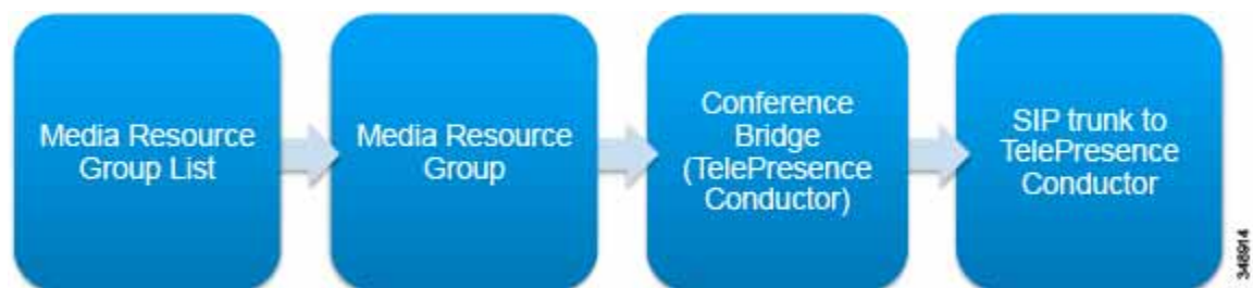
Figure 3-18 Unified CM Internal Configuration Flow for Instant Conferences
