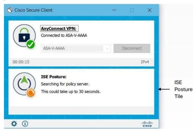
A network change starts the discovery phase. With Cisco Secure Client ISE Posture, if the default route of the primary interface is changed, it brings the agent back to the discovery process. For example, when Wi-Fi and the primary LAN are connected, the agent restarts discovery. Likewise, if Wi-Fi and the primary LAN are connected but then Wi-Fi becomes disconnected, the agent will not restart discovery.
