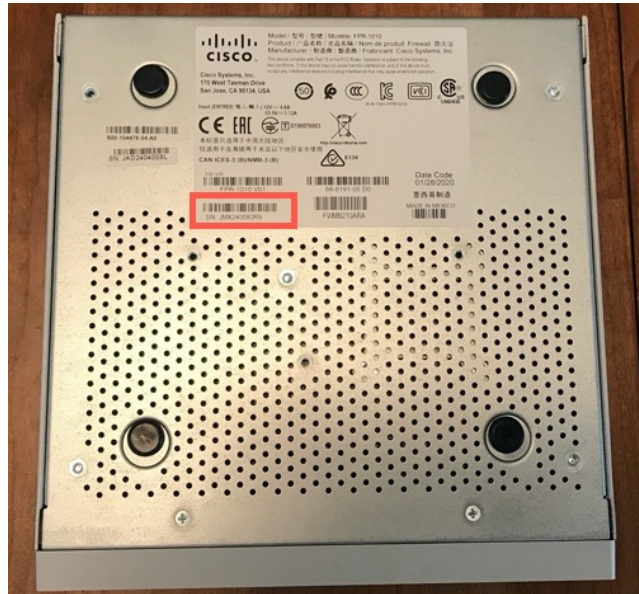
Firepower 1100: The serial number is on a label on the back of the device or on the bottom of the device.
