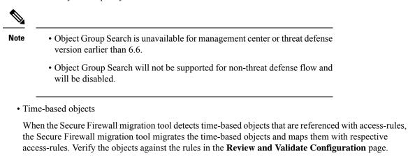
Time-based objects are access-list types that allow network access on the basis of time period. It is useful when you must place restrictions on outbound or inbound traffic on the basis of a particular time of the day or particular days of a week.
