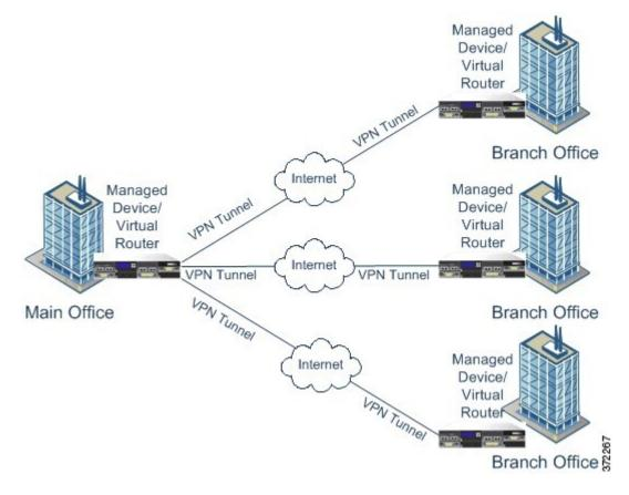
The following diagram displays a typical Hub and Spoke VPN topology.
