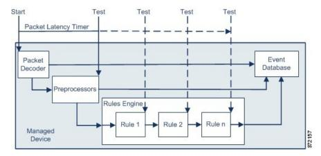
As illustrated in the above figure, packet latency timing is tested at the following test points:
